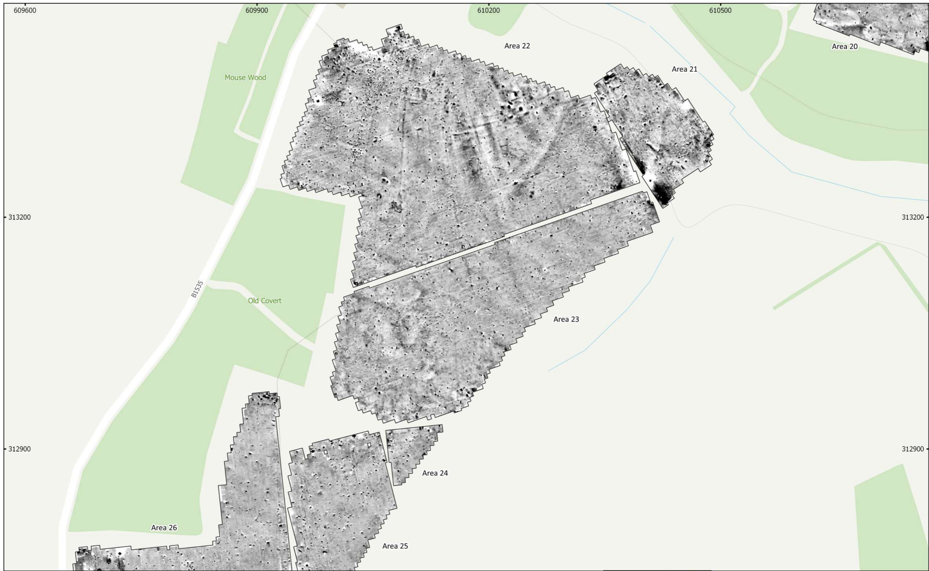
MSTG746 - Norwich Western Link Figure 18 - Magnetic Total Field (Lower Sensor)(Areas 21, 22, 23, 24, 25 & 26) 1:3,000 @ A3 Copyright Magnitude Surveys Ltd 2021 Contains Ordnance Survey data © Crown Copyright and database right 2021
